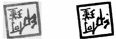
(g) 印鉴灰度图像,“印”字笔划宽度明显大于其它两个字符的笔划宽度 (h) 结构元素半径为 9 个像素长度时得到的(g)所示的灰度图像的分割结果 (g) Another original grayscale seal image, in which different characters have different stroke widths and structures (h) Thresholded top-hat result when using a disk-shaped structuring element with the radius of 9 pixels to operate the whole
