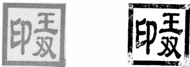
(a) 印鉴灰度图像 (b) 取半径为 10 个像素长度的圆盘形结构元素对(a)进行 top-hat 变换后,再用 Otsu 方法得到的分割结果 (a) An original grayscale seal image (b) Thresholded top-hat result of the original image in (a) when the radius of the disk-shaped structuring element is 10 pixels
