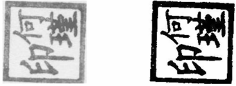
(b) 笔划分布密集的印鉴灰度图像和它的二值图像 (b) Original seal image with dense strokes and its thresholded result with poor quality
